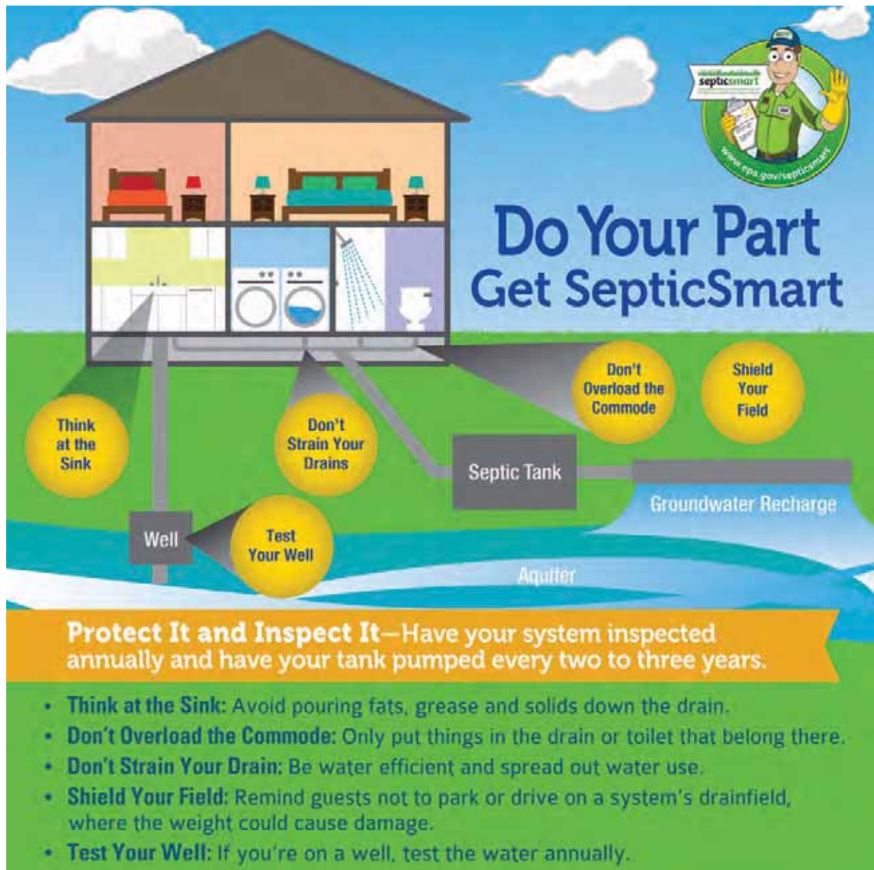
Figure 18: Environmental Protection Agency poster promoting proper septic system maintenance. Public school septic systems should be inspected annually and pumped every 2-3 years or when the total depth of the sludge and scum exceeds one third of the liquid depth of the tank.
