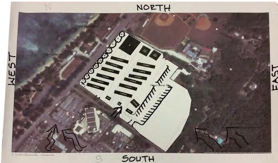
Figure 2-8 -- Wind directions are shown as wavy arrows. Parking is located at the lower flat portion. This area was identified by topographic lines as the lowest part of the site. Classrooms were aligned east-west to minimize solar heat-gain and spaced to maximize natural ventilation. Trees help reduce noise along the street.
