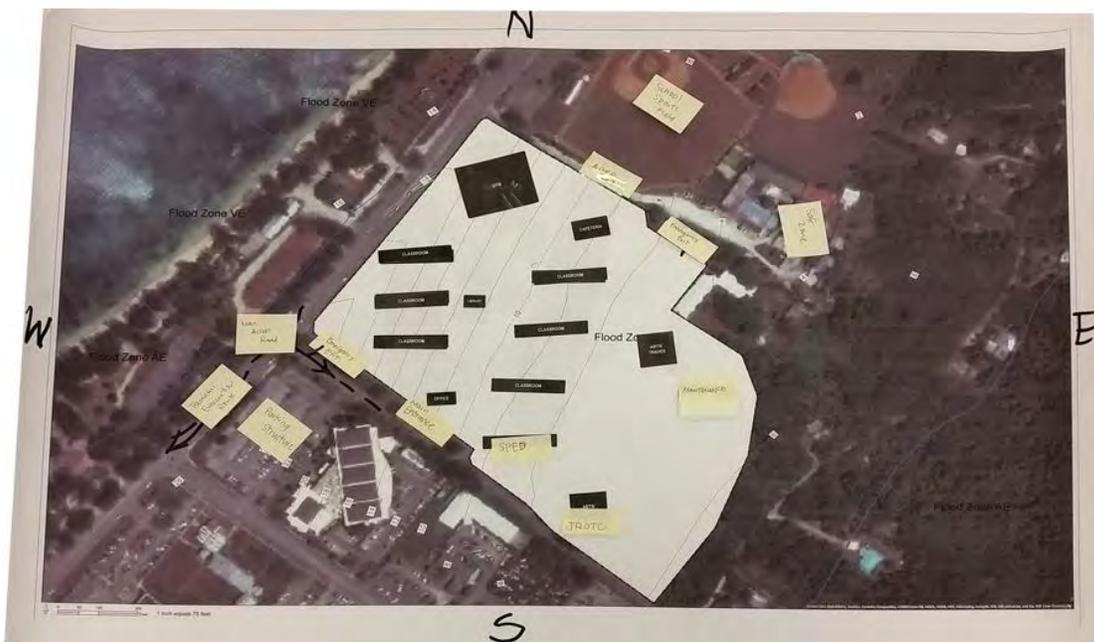
Figure 2-11 – Dashed lines at the left corner mark an Emergency Exit and Tsunami Evacuation route, which is critical for this school's close proximity to the shoreline. This site also takes advantage of an off-site parking facility, meaning the school does not need to provide/maintain a parking lot. 2-story classrooms are oriented east-west to minimize solar heat-gain and spaced to maximize natural ventilation.
