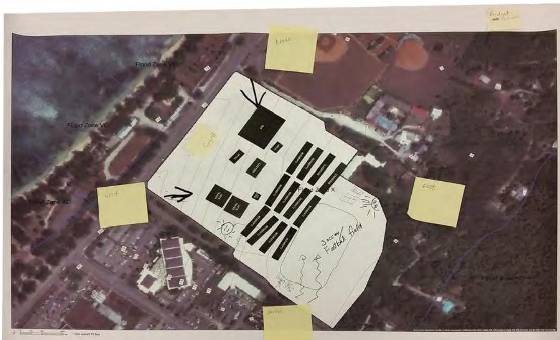
Figure 2-9 -- classroom buildings and a large soccer field are sited on the flat area of the site. The Gym (largest structure) is located adjacent to the off-site baseball and other athletic facilities. Although classrooms are not well oriented to reduce solar heat gain, they would have solar PV and be air-conditioned.
