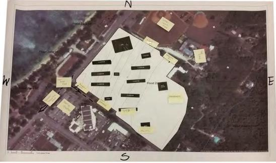
Figure 2-11 – Dashed lines at the left corner mark an Emergency Exit and Tsunami Evacuation route, which is critical for this school's close proximity to the shoreline. This site also takes advantage of an offsite parking facility, meaning the school does not need to provide/maintain a parking lot. 2-story classrooms are oriented east-west to minimize solar heat-gain and spaced to maximize vatural ventilation.
