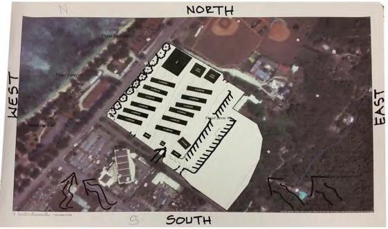
Figure 2-8 -- Wind directions are shown as wavy arrows. Parking is located at the lower flat portion. This area was identified by topographic lines as the lowest part of the site. Classrooms were aligned east-west to minimize solar heat-gain and spaced to maximize natural ventilation. Trees help reduce noise along the street.
