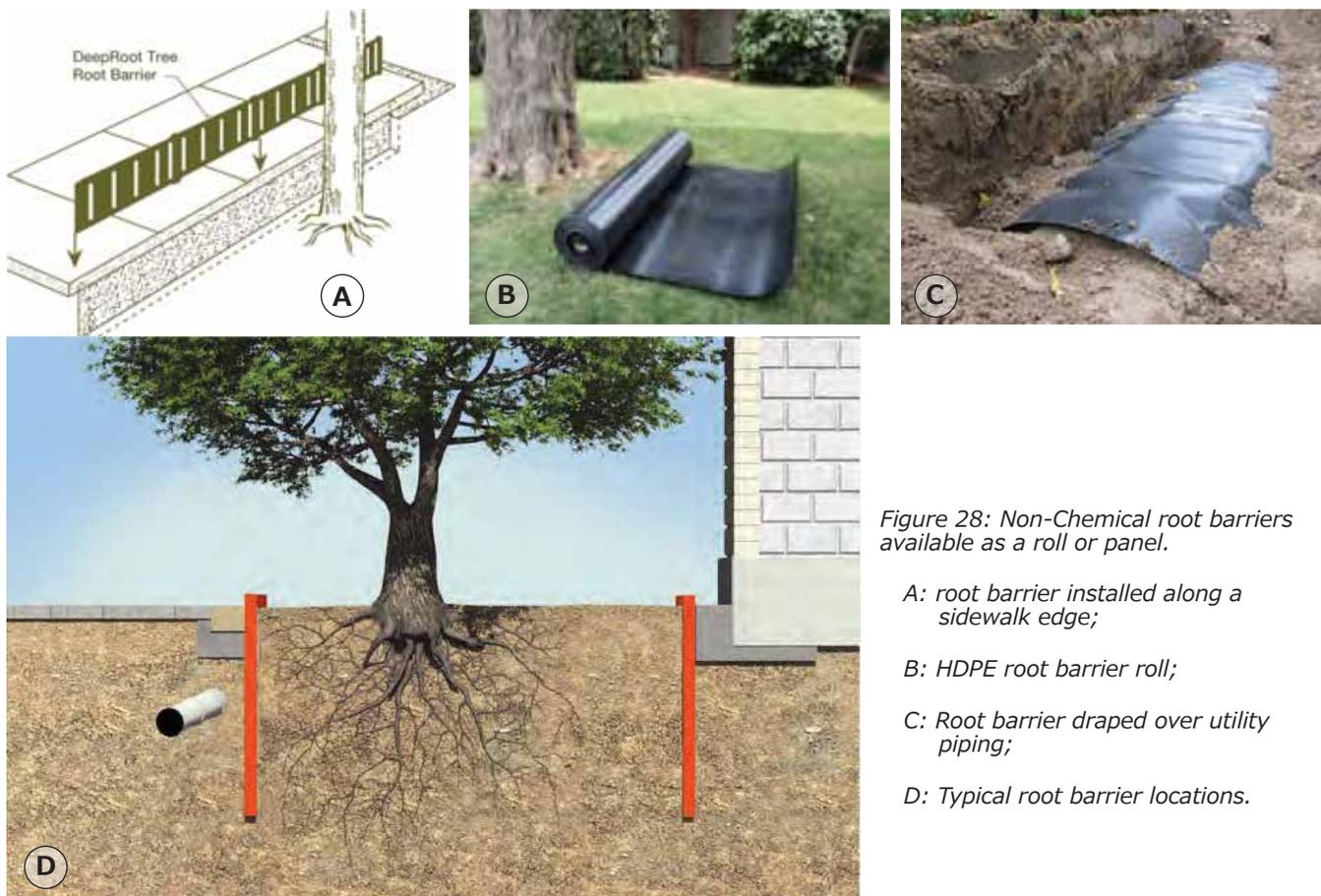
Figure 28: Non-Chemical root barriers available as a roll or panel.
