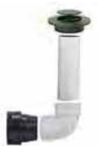
Using a Corrugated Pipe Adapter, connect the EZ-Drain to an elbow with a weep hole. The elbow should be installed with the weep hole on the horizontal side of the elbow. Slide the Pop-up Emitter onto the elbow. An additional length of pipe can be used to bring Pop-up emitter to the surface.
