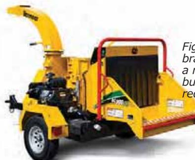
Figure 39: Chippers reduce branches and leaves into a reusable mulch product, but operating the chipper requires training.
